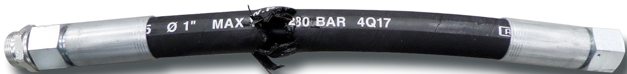
Destructive test with spiral rubber pipe 4SP DN25, according to EN 856. The pipe burst at 1480 bar, with no leaks or oozing at the sealing points.
