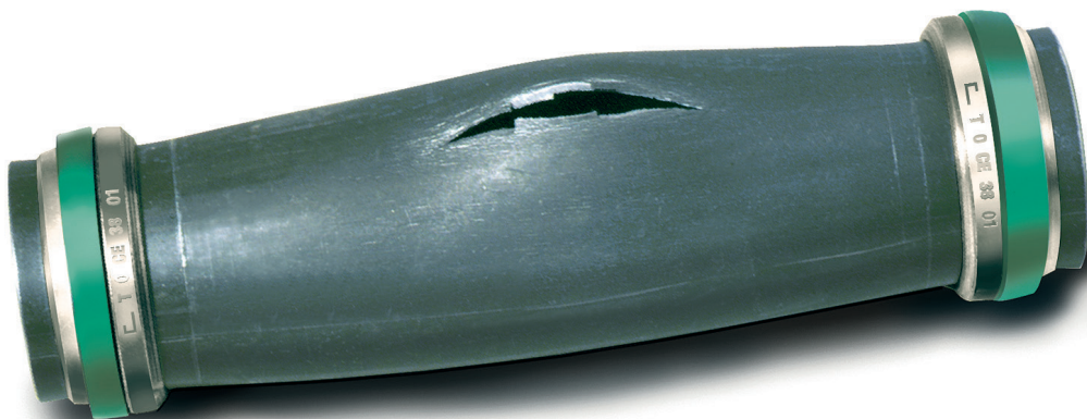
Destructive test with 28x3 carbon steel pipe. The pipe burst at 1050 bar, with no leaks or oozing at the sealing points.
